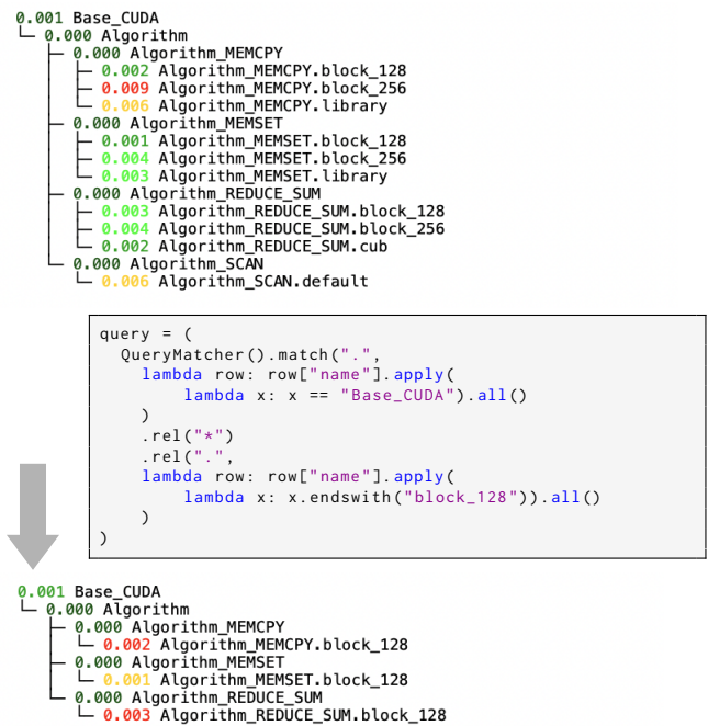
Figure 8: The call tree before (top) and after (bottom) applying the query language on a thicket object to find leaf nodes with the name ending in block_128. The call trees show the exclusive time for each node.
