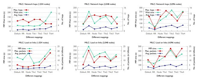
Figure 10: MILC plots comparing the time spent in point-to-point operations with average and maximum hops (top) and the MPI time with average and maximum load on network links (bottom) (Note: y-axis has a different range in each plot)
