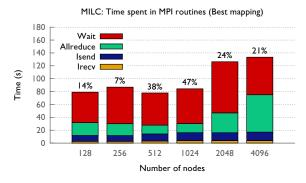
Figure 14: A scaling comparison of the benefits of task mapping for MILC on Blue Gene/Q
