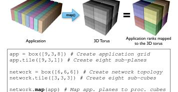
Figure 1: Mapping 2D sub-partitions to 3D shapes in Rubik
