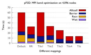
Figure 7: Average time spent in different MPI routines by pF3D on 4,096 nodes (includes MPI\_Isend optimization)
