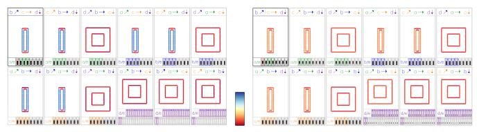
Figure 12: MILC on Blue Gene/Q: Minimaps showing aggregated network traffic along various directions for the TABCDE (left) and *Tile3* mapping (right, the colors represent aggregated traffic flowing in different directions)
