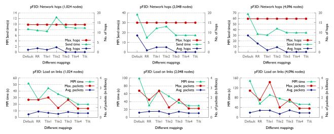
Figure 6: pF3D plots comparing the time spent in point-to-point operations with average and maximum hops (top) and the MPI time with average and maximum load on network links (bottom) (Note: y-axis has a different range in each plot)
