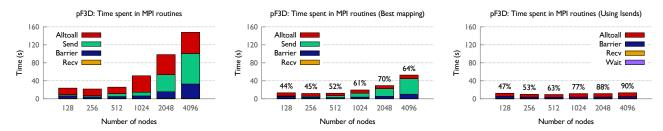
Figure 13: pF3D on Blue Gene/Q: A scaling comparison of the time spent in different MPI routines with the default mapping (left), best mapping discovered (center) and with the best mapping using the Isend optimization (right)
