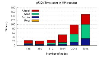
Figure 3: Average time spent in different MPI routines by pF3D for weak scaling on Blue Gene/Q
